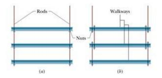
(a) In the original design, what is the total mass supported by the threads and two nuts on the lowest walkway?
